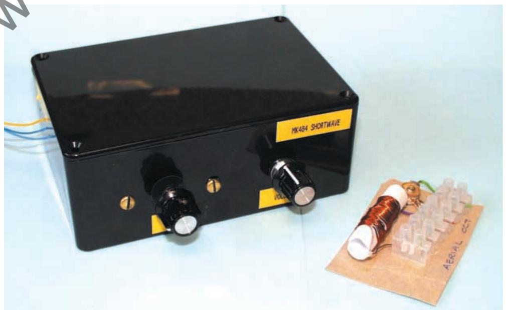
The prototype was built on a piece of stripboard measuring 50 holes by 15 copper tracks.
