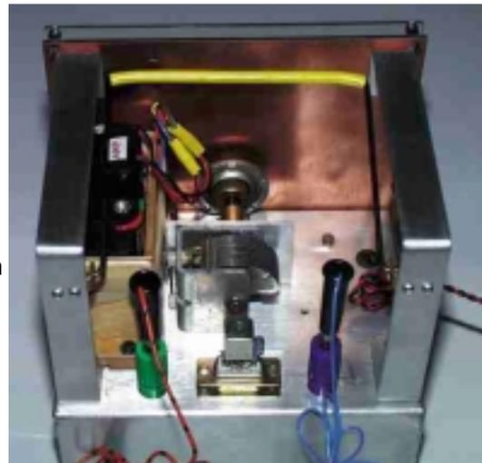
*The chassis of the prototype was fabricated from aluminum and a wooden case with hinged lid holding the loud-speaker made to house the receiver. The lid can be raised and held up by a hinged wire frame (shown above) when in use.*
