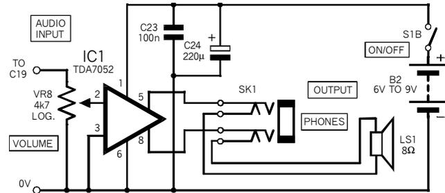
Fig 3. The audio power amplifier stage.
