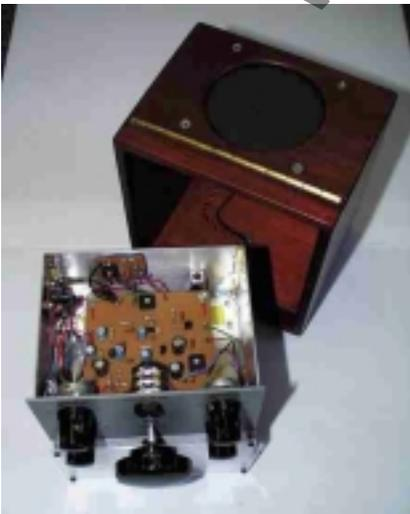
operated Bandsread control in a position remote from the tuned circuit. The prototype Receiver, shown in the photographs, incorporates this arrangement.
