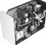
**80-132** Switch mode PSU. Nice little unit. Model No. BM43024. Input 120V AC or 240V AC. Output +5V @ 2.5A and +12V @ 2A, 36.5W. Semi-cased with mains IEC filter and switch. **£3.95**
