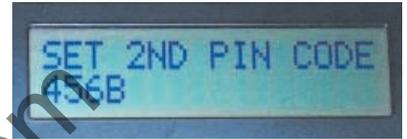
Mode 8 is used in the same way as Mode 1, but allowing you to enter the required 4-digit PIN for use with the optional keypad 2. It may be the same PIN as used with keypad 1, but it does not provide access to the main system.
