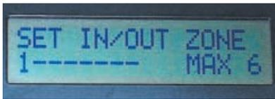
where in this instance the numeral 1 indicates that Zone 1 is currently the selected entry/exit zone. As MAX 6 states, one of six zones can be nominated as the entry/exit zone. Pressing any key between 1 and 6 selects that zone and the chosen digit appears, replacing the appropriate "dash", and with a "dash" now replacing the previous digit.
