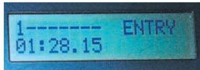
In this example, zone 1 is shown to have been entered and that it is 1 hour, 28 minutes and 15 seconds since that event. The clock continues counting until the alarm is reset via your PIN code. The elapsed time can reach 99:59:59 (just over four days – a long week-end, for example) and then restarts from zero.
