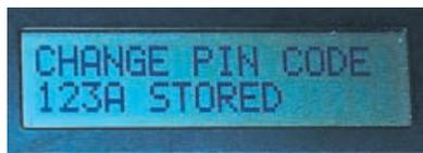
When all four digits have been entered, press D. The word STORED will now appear briefly, telling you that the code has been stored in the PIC's data EEPROM for future recall. All data EEPROM values are retained even after power has been disconnected.
