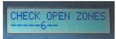
in which zone 6 is not in the required condition (e.g. a door open when it should be closed). The allocated entry/exit zone may remain open at this time, since that is the route that will be taken by the user once the alarm has been set on.
