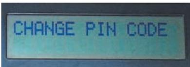
Enter your chosen 4-character PIN code using any of keys 0 to 9 and A to C, for example: 123A. The other three keys (blank, decimal point and D cannot be used for the PIN code. Each keypress is accompanied by a beep of the buzzer and its associated l.e.d. being briefly turned on.
