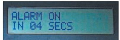
where the countdown starts at the seconds value previously set for the entry/exit delay and proceeds to count down to zero. The buzzer sounds during this period.
