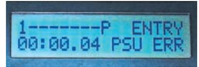
indicating that zone1 has been entered and that "panic" has been pressed, again showing the elapsed time since power restoration. The message PSU ERR (or the earlier POWER ERROR) means that you should check the condition of your battery.
