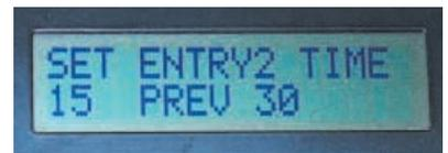
This mode sets the time during which the auxiliary output (transistor TR4) and the buzzer are activated when the correct PIN code has been keyed-in via keypad 2. At the end of the time-out, TR4 and the buzzer are turned off.
