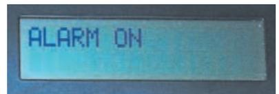
An exit from and closure of the allocated entry/exit zone must be made within the allotted entry/exit time. Failure to do so will cause an alarm condition to exist.
