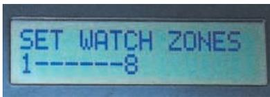
This example shows that zones 1 and 8 have been selected for unauthorised access monitoring. If any of these zones are entered when zone monitoring is active, an alarm condition will exist, accompanied by the bell and buzzer sounding, and the strobe flashing (if installed).
