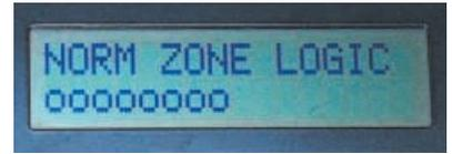
This mode is for information only. It simply shows the normally-open and normally-closed logic for each sensor as stored in the data EEPROM – in this case they are all shown as normally-open.
