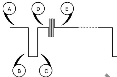
*Fig.3. Sync timing of the PIC used to clean up the output from the video recorder. (A) Enable gating to check for falling edge of line (horizontal) sync pulse. (B) Line Sync detected. Turn on IC3 to allow video sync through. (C) Turn off IC3, turn on IC4 and allow black level through. (D) Turn off IC4, turn on IC3 to allow burst through from video. (E) Turn off IC3, turn on IC4 to allow black level voltage through. Wait for approximately 60us before looping back to (A).*
