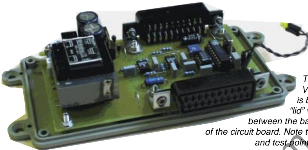
The completed PIC Video Cleaner PCB is bolted to the case "lid" with small spacers between the base and underside of the circuit board. Note the "looped" supply and test point links.
