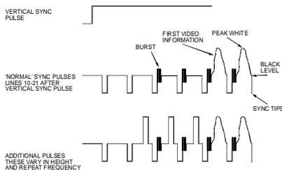
**Fig. 1. Sync pulse showing interference details.**
