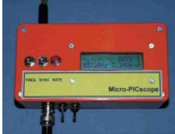
Completed *Micro-PICscope* showing general layout of display and controls.
