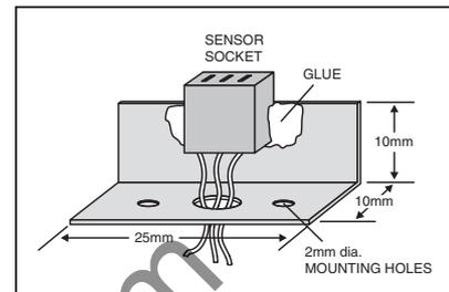
Fig.6 (right). Details of the sensor mounting bracket.
