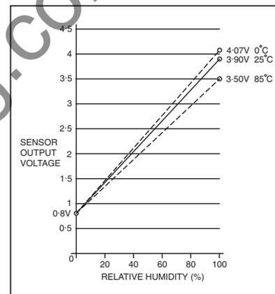
Fig. 2. HIH3605 output voltage for 0% to 100%RH.
