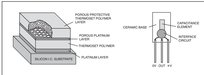
3.90V for 0%RH to 100%RH at 25°C. The change in this span with temperature is small enough to be ignored for this project, see Fig.2. For example, the 100%RH value drops to 3.50V at 85°C which is a higher temperature than likely to be encountered with this meter. But automatic temperature correction is a simple matter for high temperature applications.
