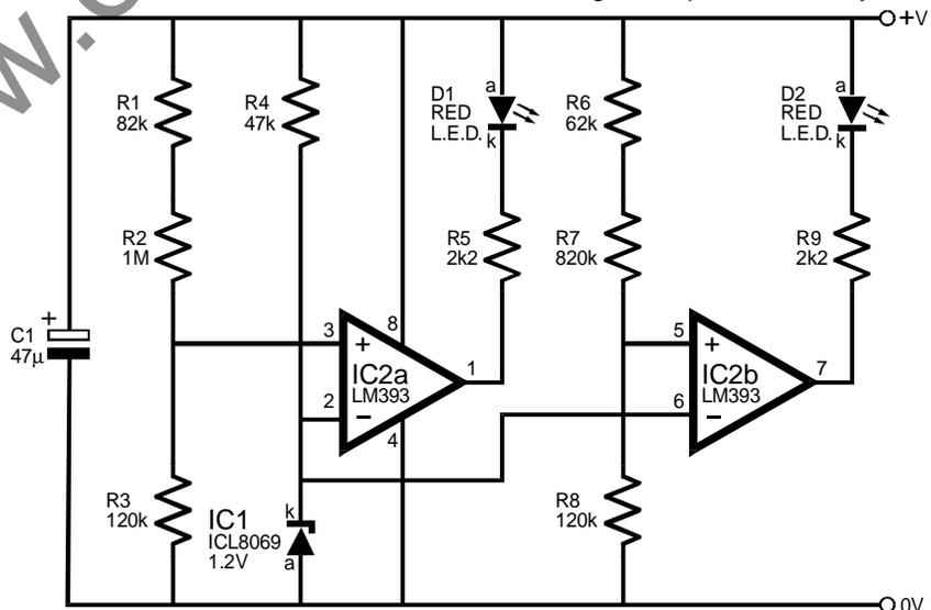
Fig. 2. Full circuit diagram for the Voltage Monitor. It is essential that an in-line fuseholder, with a 100mA fuse, is included in the positive supply input lead if the monitor is to be installed in a car, boat, caravan etc.
