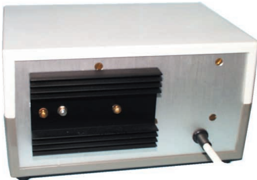
Rear of the completed power supply unit showing the finned heatsink bolted to the rear panel to aid dissipation of heat from the power MOSFET.
