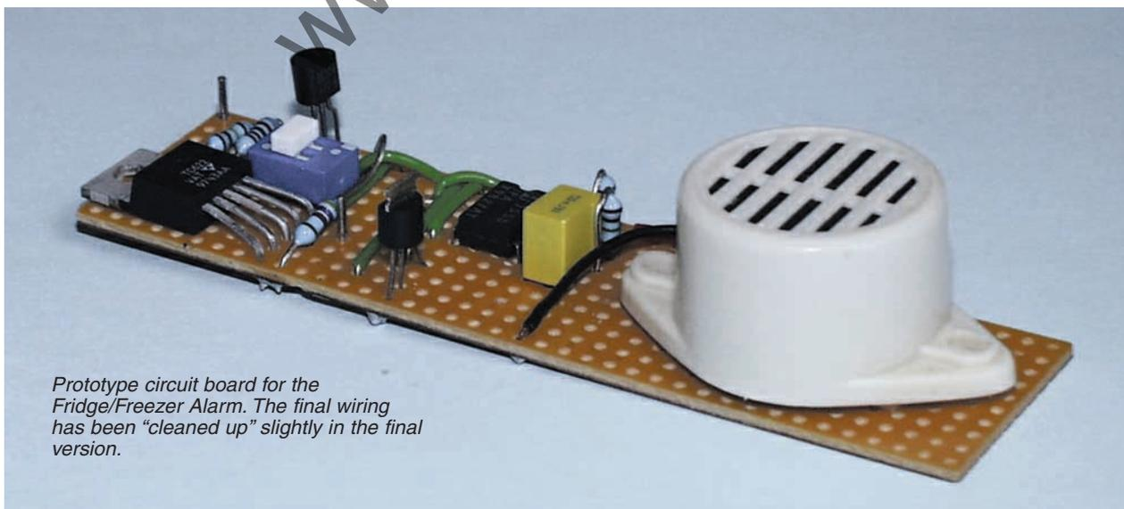
Prototype circuit board for the Fridge/Freezer Alarm. The final wiring has been "cleaned up" slightly in the final version.
