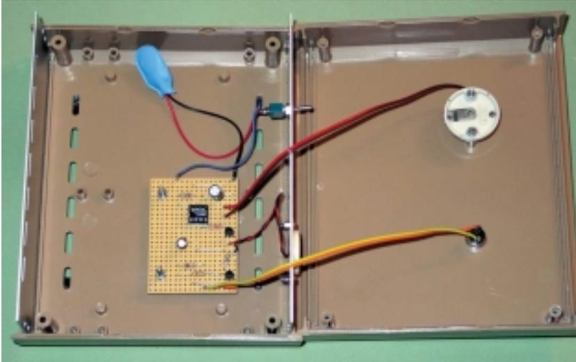
*The two halves of the case opened out to reveal the general positioning of the circuit board and the interwiring to the front and top panel mounted components. Don't forget to leave plenty of room for the battery.*
