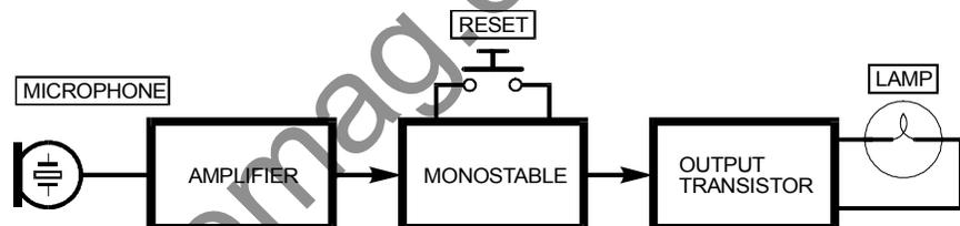
Fig. 1. Block diagram for the Automatic Nightlight.
