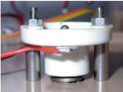
*Using spacers to mount the bulb holder on the underside of the case lid, above a 9mm diameter hole to allow the bulb to be screwed in from the outside.*
