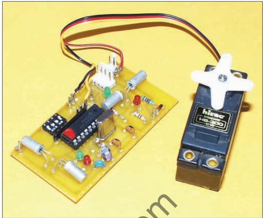
Completed printed circuit board connected to a single servo motor. Note the four attitude tilt switches.
