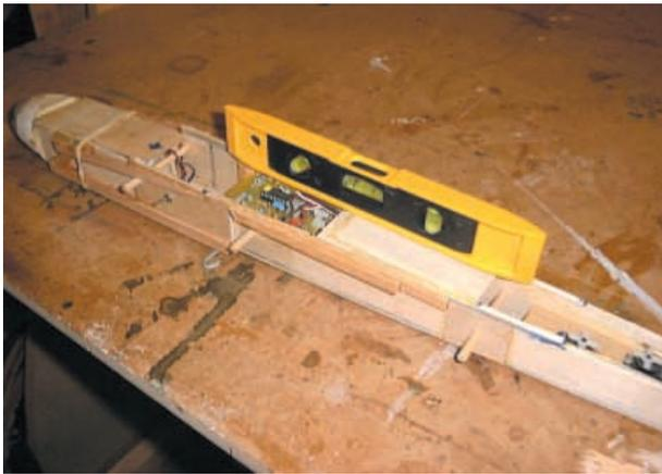
Using a spirit level to check fuselage "balance".
