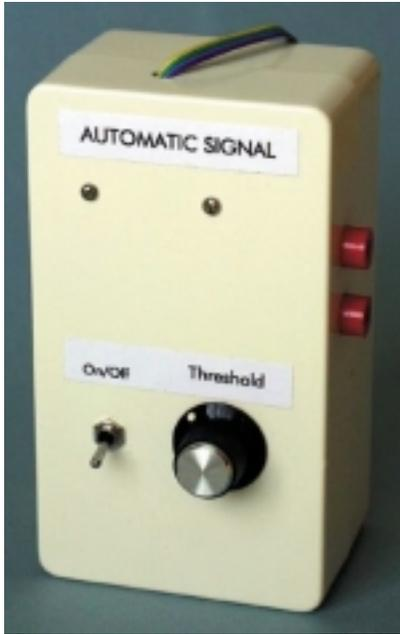
never produce an output level that is right down at zero volts, and the threshold level must be high enough to ensure that the signal does go to red when the train stops.
