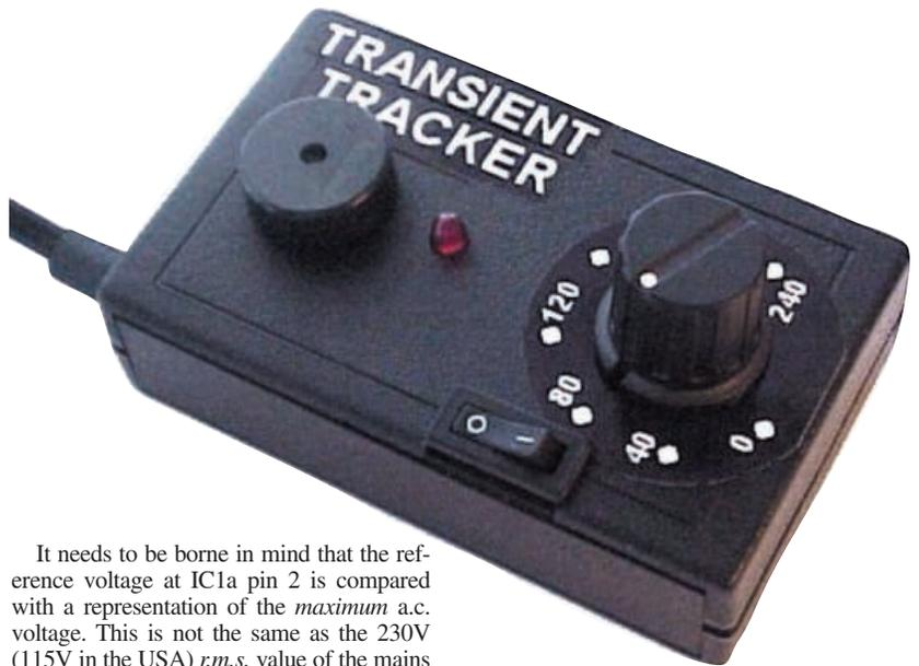
It needs to be borne in mind that the reference voltage at IC1a pin 2 is compared with a representation of the *maximum* a.c. voltage. This is not the same as the 230V (115V in the USA) *r.m.s.* value of the mains voltage. The *r.m.s.* value is multiplied by the square root of 2 to obtain the maximum value, which is 325V (163V in the USA).
