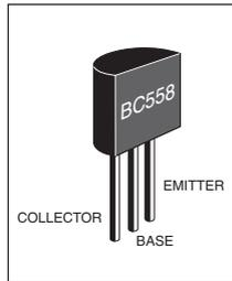
TR1 is a *npn* device and although a BC558 has been specified, virtually any small *npn* device can be used.
