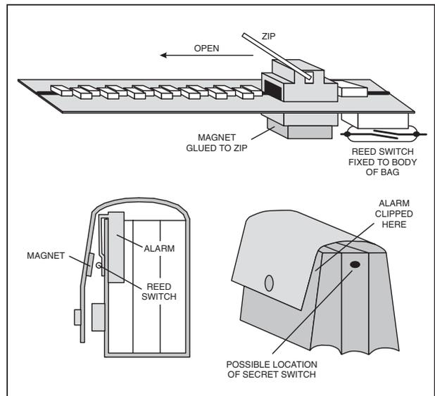
Fig.1. Some suggested ideas on how and where to mount the Pickpocket Alarm. The photograph on the left shows the reed switch mounted on the "pocket clip" and a small magnet to one side of the case.
