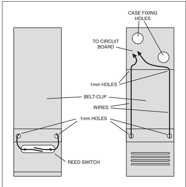
Fig.6. One suggested method of mounting and wiring the magnet-operated reed switch on the case belt-clip.
