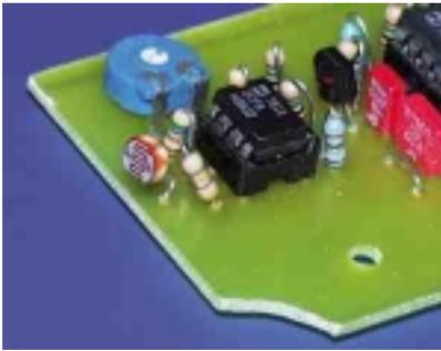
Close-up of circuit board showing the leads of the LDR carefully bent at right-angles to the PCB to align with "light window" in side of case.
