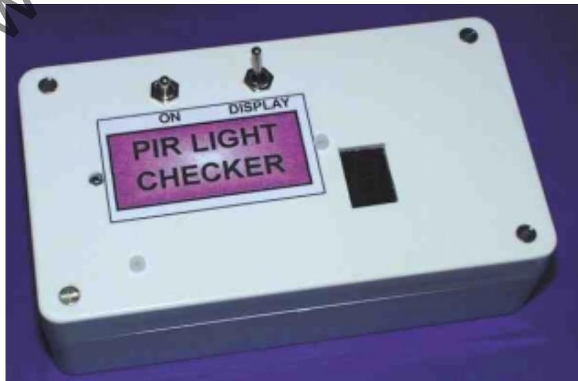
*Completed PIR Light Checker front panel layout.
