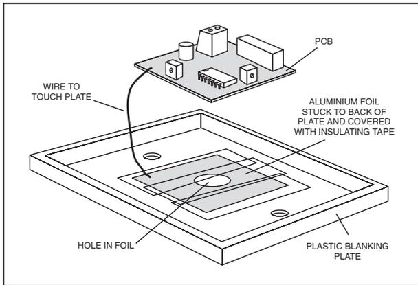
Fig.5. Suggested touch switch assembly.
