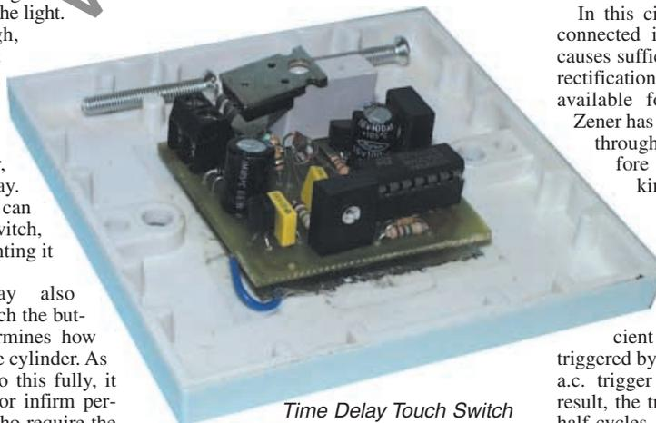
*Time Delay Touch Switch mounted on the rear of an electrical blanking plate.*
