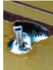
A "dry" joint. Solder failed to flow.
