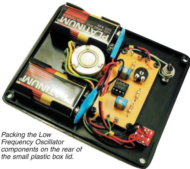
Packing the Low Frequency Oscillator components on the rear of the small plastic box lid.
