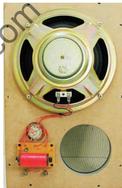
Main speaker and crossover filter (last month) mounted on the rear of the enclosure front panel.
