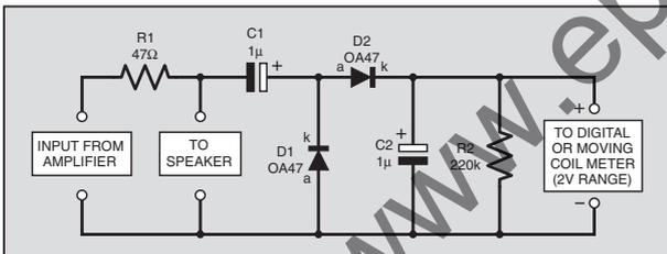
Fig.6. Circuit diagram for the loudspeaker Resonance Detector.
