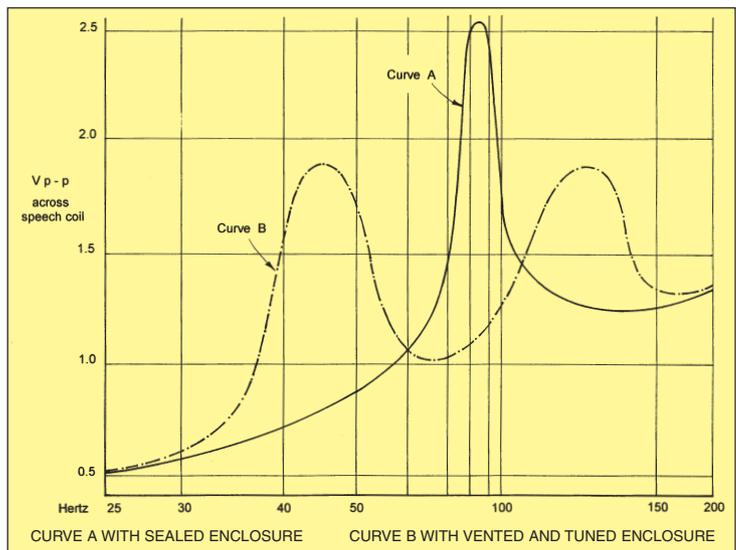
Fig. 1. Speech coil impedance in region of resonance.
