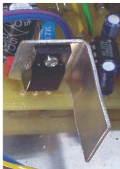
Close-up detail of heatsink mounted on IC3.
