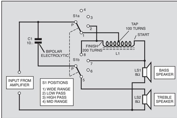
Fig.6. Circuit diagram for the Loudspeaker Crossover/Audio Filter.
