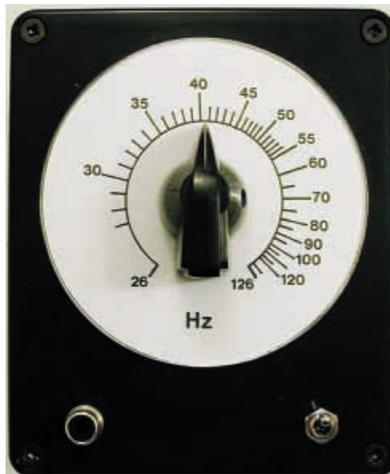
Low Frequency Oscillator for loud-speaker resonance checking.
