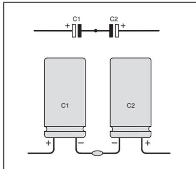
Fig.5. Creating a bipolar electrolytic from two capacitors.
