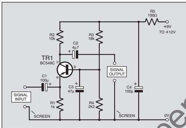
VOLTAGE GAIN 100 OVER AN  $h_{fe}$  SPREAD OF 110 TO 600.
