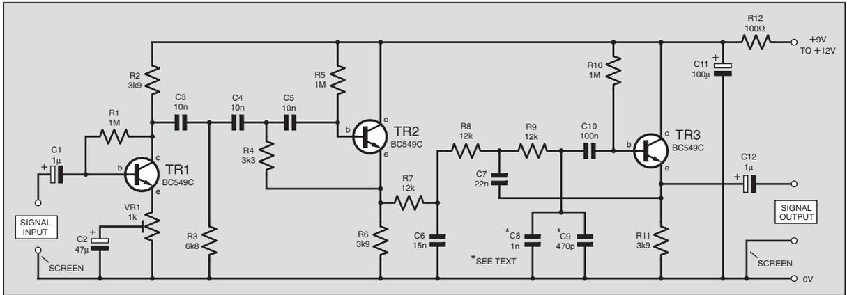
VOLTAGE GAIN WITH PASSBAND, UNITY WITH VR1 SLIDER AT 0V RAIL; 25 WITH SLIDER AT TR1 EMITTER END.
