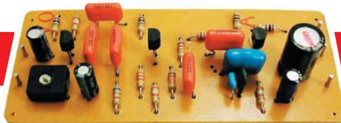
Bandpass Filter printed circuit board.
