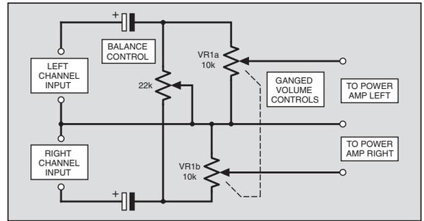
Fig. 16. Circuit arrangement for a stereo Balance control.
