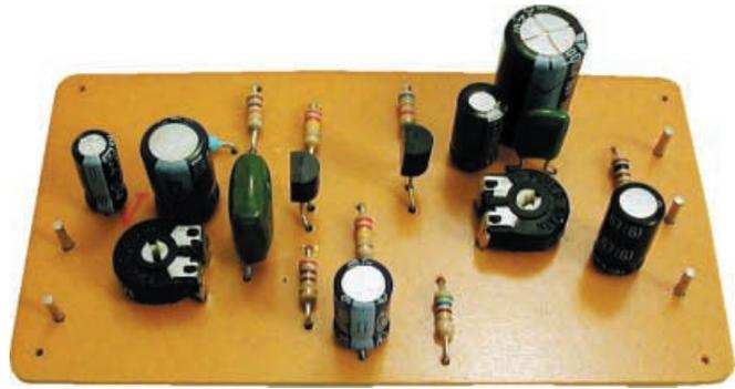
Completed p.c.b. for the Low-Noise Preamplifier.
