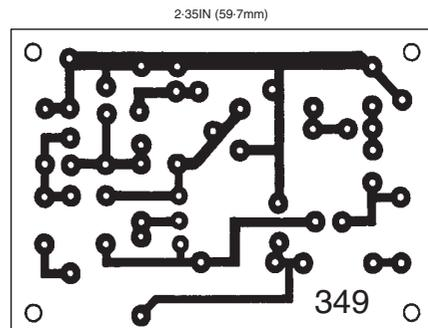
Fig.8. Printed circuit board component layout, wiring and full-size copper foil master for the F.E.T. High Input Impedance Preamp.
