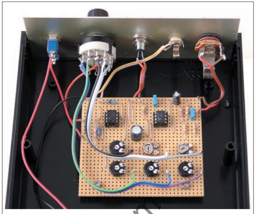
*Interwiring from the circuit board to the front panel mounted components.*
